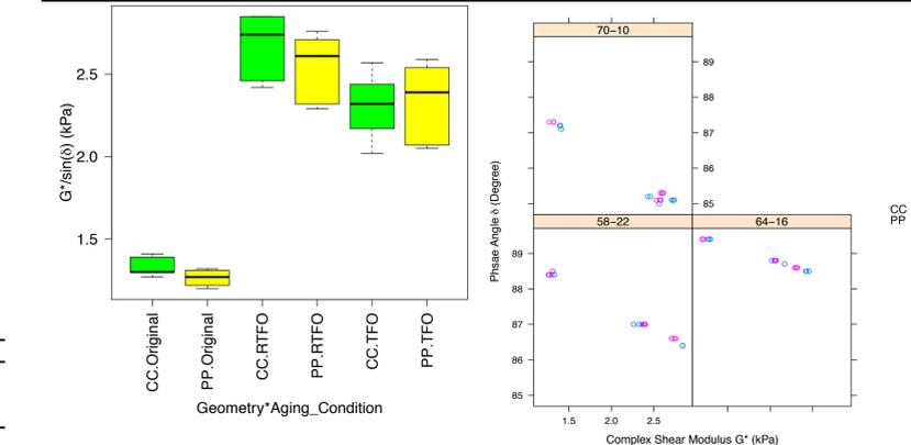
FIGURE 5a:  $G^*/\sin(\delta)$  with fixed conversion factor at 58°C, 64°C, and 70°C on unaged and aged binders.
